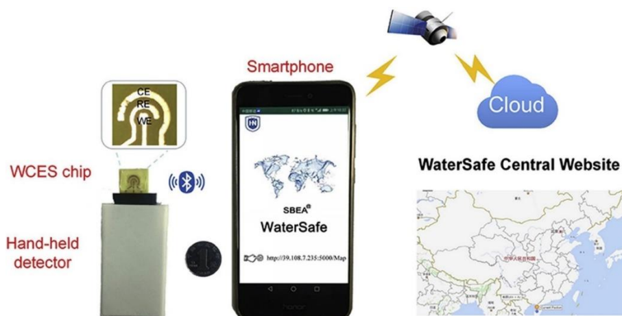
Figure 6. Smartphone-Based Water Quality Monitoring System (Liao et al., 2020)
